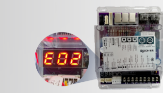
Error self-check program Service engineer can be quickly identify the faults according to error code for high efficient maintenance
